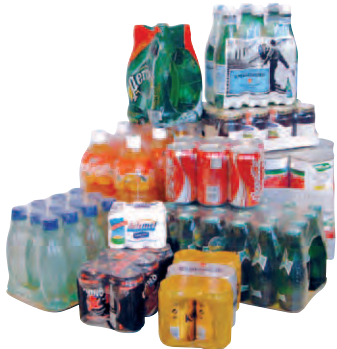
Packs in shrink film wrapping made with the LSK (SMI).
