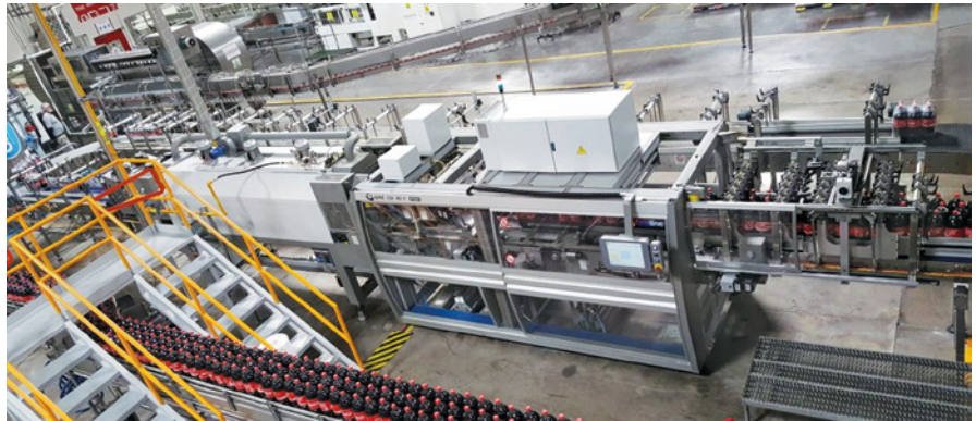
CSK 40 compact packer equipped with a methane gas shrink-tunnel (SMI).
