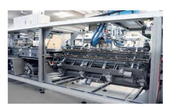
it is possible to obtain different pack configurations with the CM R combined packer. All this without any mechanical adjustment to be manually made by the operator.
