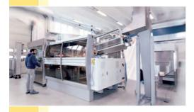
The EBS K Ergon stretch-blow moulder is available in 2, 3 and 4-cavity versions. It is claimed to offer the advantages of rotary technology in a speed range (from 1,000 to 9,000 bph) that is traditionally served by linear stretch-blow moulders.
