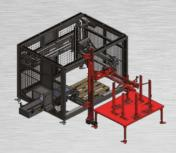
The pad-inserting module is a pad feeding system adjustable according to the different size of the interlayer pad, that can be matched to the structure of the palletizer. The suction-cup gripping system with 4 adjustable points ensures the accurate lifting of any kind of interlayer pad. The loading of the pads
