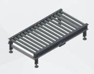
Painted steel frame. Rollers with 76 mm Ø and 150 mm pitch, motorized through a 5/8 inch chain. Electronically reversible central motorization. The system is controlled by the main electrical cabinet. Designed in accordance with FCR (Full Cost Reduction) it is tested and supplied to the customer completely mounted and cabled.
