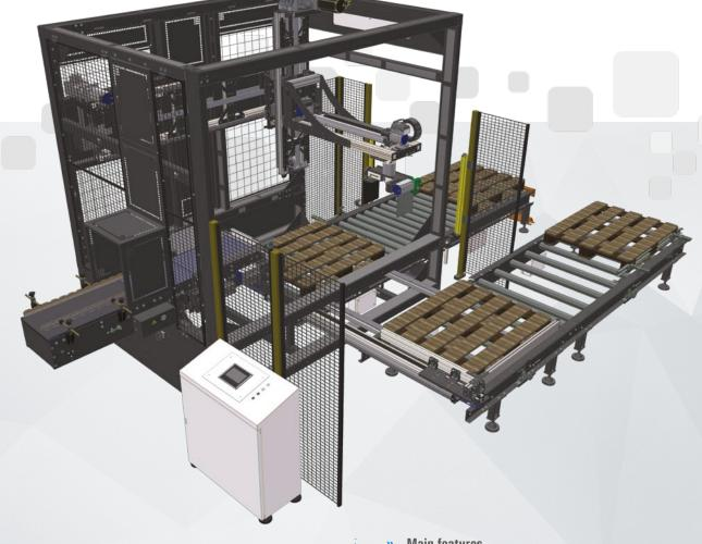
Later, it is brought into the picking position by a distancing conveyor, where the gripping head picks the pack, individually or grouped, and places it on the pallet fed by specific roller conveyors.
