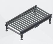
Painted steel frame. Rollers with 76 mm Ø and 150 mm pitch, motorized through a 5/8 inch chain. Electronically reversible central motorization. The system is controlled by the main electrical cabinet. Designed in accordance with FCR (Full Cost Reduction) it is tested and supplied to customer completely mounted and cabled.
