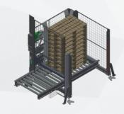
empty pallets Maximum height: 1800 mm Pile maximum weight: 300 kg
