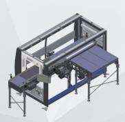
Single-entry infeed with 90° layer-forming system equipped with: 1 rubberized cadencing belt, 1 product infeed belt, in order to form the row and 1 onetranslation system that contributes to forming the layer into the basket. The layer-forming system is equipped with energyefficient motors. Designed
