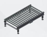
Frame in painted steel and rollers with 76 mm ø 150 mm pitch, motorised through a 5/8 inch chain. Electronically reversible central motorization. The system is tested in SMI factory and is supplied to the client fully assembled and cabled. Available in different lengths: 1500 mm, 2000 mm, 2500 mm and 3000 mm.
