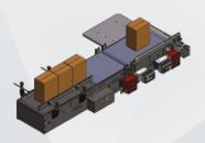
The product arriving at the palletizer is cadenced by the rubber conveyor. The distancing conveyor moves the product to the picking position (depending on the product size and palletizing pattern
