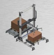
The pad-inserting module is a pad feeding system adjustable in accordance with the size of the interlayer pad, that can be combined with the central column of the APS ERGON palletizer. Suction-cup gripping system from 4 up to 8 adjustable points to ensure the accurate lifting of any kind of interlayer. The interlayer pad automatic loading is available as optional
