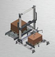
The pad-inserting module is a pad feeding system adjustable in accordance with the size of the interlayer pad, that can be combined the central column of the APS ERGON palletizer. Suctioncup gripping system from 4 up to 8 adjustable points to ensure the accurate lifting of any kind of interlayer. The interlayer pad automatic loading is available as optional and allows to load the pallet
