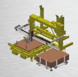
With high machine cycles, in case the pad needed not only between the layers, but also on the pallet, the new accessory "inserting the first pad" is required.
