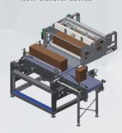
row transfer process is managed by a motorized bar. After a row is formed, it gets pushed straight away into the loading head (basket). The system is equipped a "dead" plate (buffer), which enables to continue with the row push-in operations even when the head is not yet in the loading position.
