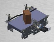
This optional system allows to turn packs being fed to the palletizer by means of a contrast cylinder. If packs get to the machine with the short side leading, a second optional cylinder is available to ease the rotation process.
