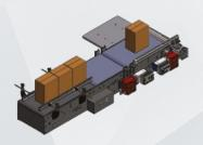
The product arriving at the palletizer is cadenced by the rubber conveyor. The distancing conveyor moves the product to the picking position (depending on the product size and palletizing pattern required, even more products can be
