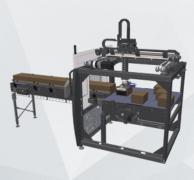
By means of an innovative system of pack rotation and/ or manipulation in continuous motion on three Cartesian axes (x, y and z), bundles coming along a belt in single (APS 3070 L) or double (APS 3105 L e 3140 L) lane are turned, shifted and arranged onto
