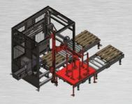
The pad-inserting module is a pad feeding system adjustable according to the different size of the interlayer pad, that can be matched to the structure of the palletizer. The suctioncup gripping system with 4 adjustable points ensures the accurate lifting of any kind
