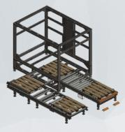
The empty pallet, after having been loaded in the position external to the nets, is automatically brought into the pallet formation area. The pallet 90° transfer is ensured by a pneumatic device (Devio), that, moves the pallet to the desired position thanks to a cylinder. The full pallet is moved to the roller
