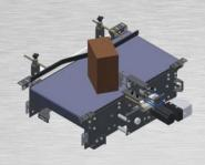
This optional system allows to turn packs being fed to the palletizer by means of a contrast cylinder. If packs get to the machine with the short side leading, a second optional cylinder is available to ease the rotation process.
