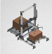
The pad-inserting module is a pad feeding system adjustable in accordance with the size of the interlayer pad, that can be combined with the central column of the APS ERGON palletizer. Suction-cup gripping system from 4 up to 8 adjustable points to ensure the accurate lifting of any kind of interlayer. The interlayer pad automatic loading is available
