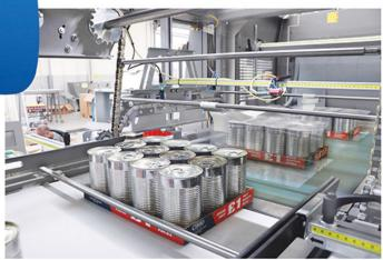
The two rotary modules are supplied with double equipment: (a) that required for working in film only and (b) that for packaging in tray or wraparound boxes.
